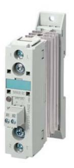
SEMI-COND. CONTACTOR 3RF2,1-PH. AC 51 10 A / AC15 6A 40 DEG. C 24-230 V / 110-230 V AC INSTANTANEOUS SWITCHING
