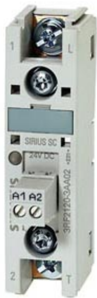
SEMICONDUCTOR RELAY 3RF2, 1-PH. WIDTH 22.5MM, 50 A 48-460 V / 24 V DC RING TERMINAL
