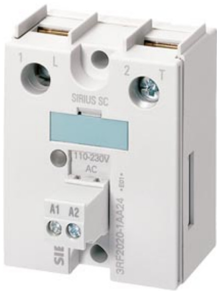
SEMICONDUCTOR RELAY 3RF2, 1-PH. WIDTH 45MM, 70 A 48-600 V / 110-230 V AC SCREW TERMINAL
