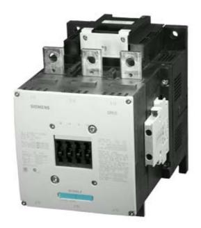
CONTACTOR, 690A/AC-1 AC(40...60HZ)/DC OPERATION UC 220-240V AUXILIARY CONTACTS 2NO+2NC 3-POLE, SIZE S12 BAR CONNECTIONS CONVENT. OPERATING MECHANISM
