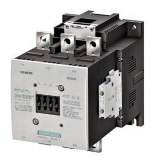
CONTACTOR, 690A/AC-1 AC(40...60HZ)/DC OPERATION UC 200-220V AUXILIARY CONTACTS 2NO+2NC 3-POLE, SIZE S12 BAR CONNECTIONS CONVENT. OPERATING MECHANISM
