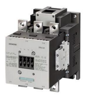
CONTACTOR, 400A/AC-1 AC(40...60HZ)/DC OPERATION UC 220-240V AUXILIARY CONTACTS 2NO+2NC 3-POLE, SIZE S10 BAR CONNECTIONS CONVENT. OPERATING MECHANISM
