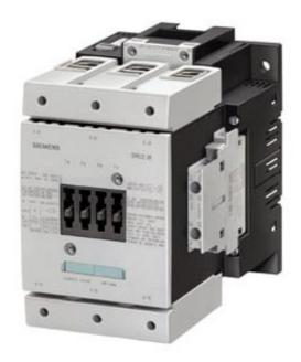
CONTACTOR, 275A/AC-1, AC(40...60HZ)/DC OPERATION UC 440...480V AUXIL. CONTACTS 2NO+2NC 3-POLE, SIZE S6 BAR CONNECTIONS CONVENT. OPERATING MECHANISM
