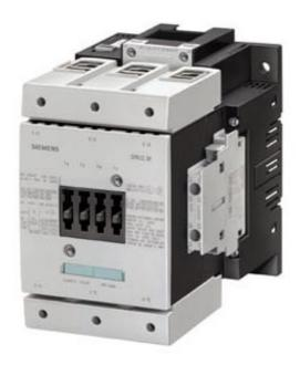
CONTACTOR, 275A/AC-1, AC(40...60HZ)/DC OPERATION UC 220...240V AUXIL. CONTACTS 2NO+2NC 3-POLE, SIZE S6 BAR CONNECTIONS CONVENT. OPERATING MECHANISM
