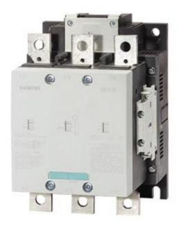
VAC. CONTACTOR, 110KW/400V/AC-3 AC(40...60HZ)/DC OPERATION UC 380-420V AUXILIARY CONTACTS 2NO+2NC 3-POLE, SIZE S10 BAR CONNECTIONS CONVENT. OPERATING MECHANISM
