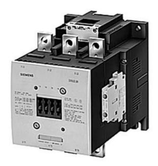
CONTACTOR, 250KW/400V/AC-3 AC(40...60HZ)/DC OPERATION UC 200-277V AUXILIARY CONTACTS 2NO+2NC 3-POLE, SIZE S12 BAR CONNECTIONS ELECTRONIC OPERATING MECHANISM WITH 24V DC PLC INTERFACE SCREW TERMINAL
