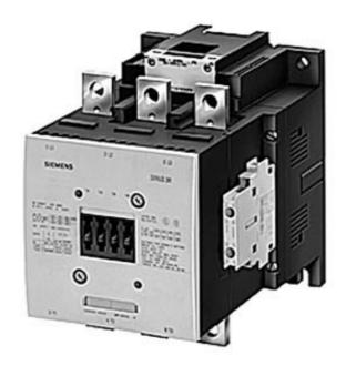
CONTACTOR, 250KW/400V/AC-3 AC(40...60HZ)/DC OPERATION UC 220-240V AUXILIARY CONTACTS 2NO+2NC 3-POLE, SIZE S12 BAR CONNECTIONS CONVENT. OPERATING MECHANISM SCREW TERMINAL
