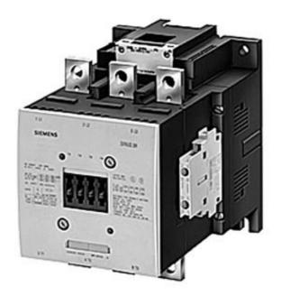
CONTACTOR, 250KW/400V/AC-3 AC(40...60HZ)/DC OPERATION UC 380-420V AUXILIARY CONTACTS 2NO+2NC 3-POLE, SIZE S12 BAR CONNECTIONS CONVENT. OPERATING MECHANISM SCREW TERMINAL
