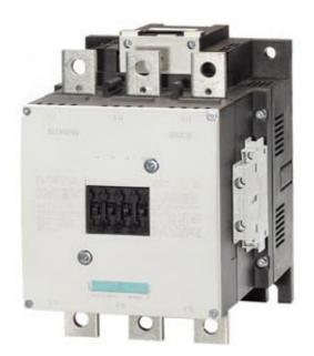
CONTACTOR, 200KW/400V/AC-3 AC(40...60HZ)/DC OPERATION UC 200-277V AUXILIARY CONTACTS 2NO+2NC 3-POLE, SIZE S12 BAR CONNECTIONS ELECTRONIC OPERATING MECHANISM WITH 24V DC PLC INTERFACE SCREW TERMINAL
