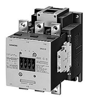
CONTACTOR, 160KW/400V/AC-3 AC(40...60HZ)/DC OPERATION UC 220-240V AUXILIARY CONTACTS 2NO+2NC 3-POLE, SIZE S10 BAR CONNECTIONS CONVENT. OPERATING MECHANISM SCREW TERMINAL
