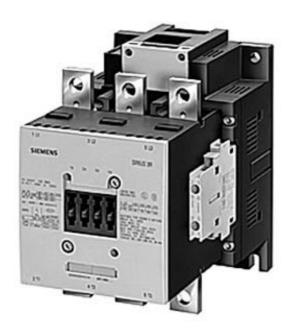
CONTACTOR, 160KW/400V/AC-3 AC(40...60HZ)/DC OPERATION UC 200-220V AUXILIARY CONTACTS 2NO+2NC 3-POLE, SIZE S10 BAR CONNECTIONS CONVENT. OPERATING MECHANISM SCREW TERMINAL
