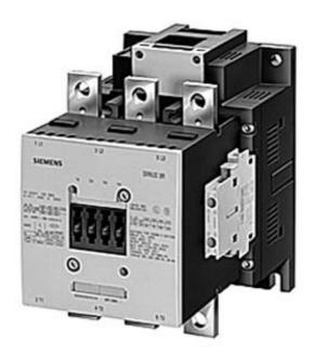
CONTACTOR, 132KW/400V/AC-3 AC(40...60HZ)/DC OPERATION UC 96-127V AUXILIARY CONTACTS 2NO+2NC 3-POLE, SIZE S10 BAR CONNECTIONS ELECTRONIC OPERATING MECHANISM WITH 24V DC PLC INTERFACE SCREW TERMINAL
