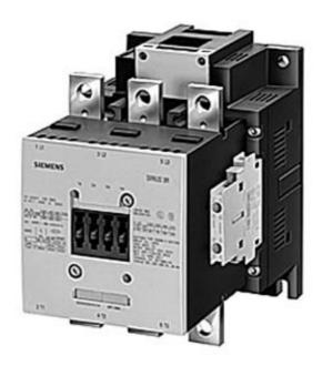
CONTACTOR, 132KW/400V/AC-3 AC(40...60HZ)/DC OPERATION UC 21-27.3V AUXILIARY CONTACTS 2NO+2NC 3-POLE, SIZE S10 BAR CONNECTIONS ELECTRONIC OPERATING MECHANISM WITH 24V DC PLC INTERFACE SCREW TERMINAL
