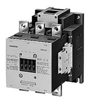
CONTACTOR, 132KW/400V/AC-3 AC(40...60HZ)/DC OPERATION UC 500-550V AUXILIARY CONTACTS 2NO+2NC 3-POLE, SIZE S10 BAR CONNECTIONS CONVENT. OPERATING MECHANISM SCREW TERMINAL
