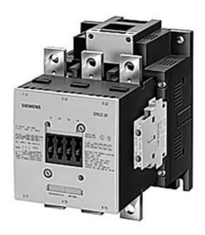
CONTACTOR, 110KW/400V/AC-3 AC(40...60HZ)/DC OPERATION UC 23-26V AUXILIARY CONTACTS 2NO+2NC 3-POLE, SIZE S10 BAR CONNECTIONS CONVENT. OPERATING MECHANISM SCREW TERMINAL
