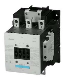
CONTACTOR, 90KW/400V/AC-3, AC(40...60HZ)/DC OPERATION UC 440...480V AUXIL. CONTACTS 2NO+2NC 3-POLE, SIZE S6 BAR CONNECTIONS CONVENT. OPERATING MECHANISM SCREW TERMINAL
