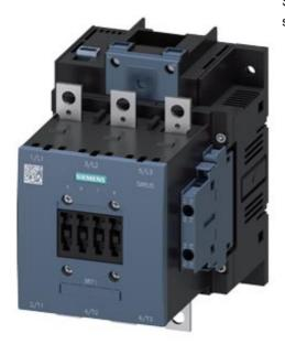
Power contactor, AC-3 150 A, 75 kW / 400 V AC (50-60 Hz) / DC operation 21-27 UC, 3 V Auxiliary contacts 2 NO + 2 NC 3-pole, Size S6 Busbar connections Drive: electronic with PLC interface 24 V DC screw terminal
