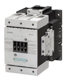
CONTACTOR, 55KW/400V/AC-3 AC(40...60HZ)/DC OPERATION UC 200...277V AUXIL. CONTACTS 2NO+2NC 3-POLE, SIZE S6 WITH BOX TERMINALS ELECTRONIC OPERATING MECHANISM WITH PLC INTERFACE 24V DC SCREW TERMINAL
