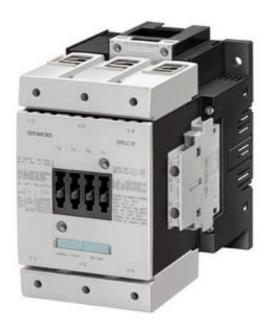
CONTACTOR, 55KW/400V/AC-3 AC(40...60HZ)/DC OPERATION UC 21...27,3V AUXIL. CONTACTS 2NO+2NC 3-POLE, SIZE S6 WITH BOX TERMINALS ELECTRONIC OPERATING MECHANISM WITH PLC INTERFACE 24V DC SCREW TERMINAL
