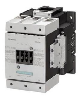
CONTACTOR, 55KW/400V/AC-3, AC(40...60HZ)/DC OPERATION UC 240...277V AUX. CONTACTS 2NO+2NC, 3-POLE, SIZE S6 WITH BOX TERMINALS CONVENTIONAL OPERATING MECHAN. SCREW TERMINAL
