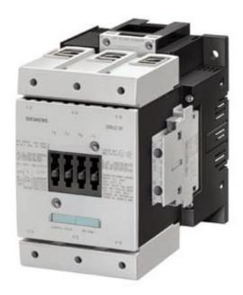
CONTACTOR, 55KW/400V/AC-3 AC(40...60HZ)/DC OPERATION UC 200...220V AUXIL. CONTACTS 2NO+2NC 3-POLE, SIZE S6 WITH BOX TERMINALS CONVENTIONAL OPERATING MECHAN. SCREW TERMINAL
