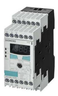
TEMPERATURE MONITORING RELAY PT100/500/1000 KTY83/84, NTC 2 THRESH. VAL., DIGITAL -50 C - 500 C, 24V AC/DC 2 X 1 W + 1 NO, WIDTH 45 MM SCREW CONNECTION
