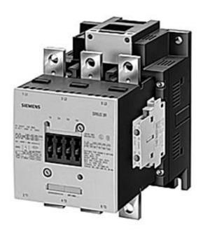
CONTACTOR, 110KW/400V/AC-3 AC(40...60HZ)/DC OPERATION UC 220-240V AUXILIARY CONTACTS 2NO+2NC 3-POLE, SIZE S10 BAR CONNECTIONS CONVENT. OPERATING MECHANISM SCREW TERMINAL
