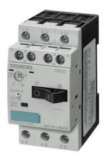
CIRCUIT-BREAKER SIZE S00, FOR MOTOR PROTECTION, CLASS 10, A-REL. 7...10A, N-REL. 130A, SCREW TERMINAL, STANDARD SWITCHING CAPACITY, W. TRANSV. AUX. SWITCH 1NO/1NC
