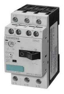
CIRCUIT-BREAKER, SIZE S00, FOR MOTOR PROTECTION, CLASS 10, A REL.5.5...8 A, N REL.104 A, 1NO + 1NC TRANSVERSE, SCREW CONN., STANDARD BREAKING CAPAC.
