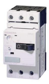
CIRCUIT-BREAKER, SIZE S00, FOR MOTOR PROTECTION, CLASS 10, A REL.0.11...0.16A, N REL.2.1A SCREW CONNECTION, STANDARD BREAKING CAPACITY, W. TRANSV. AUX. SWITCH 1NO/1NC
