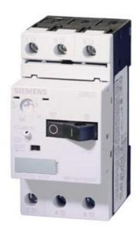
CIRCUIT-BREAKER, SIZE S00, FOR MOTOR PROTECTION, CLASS 10, A REL. 0.70...1A, N REL. 13A, SCREW CONNECTION, STANDARD BREAKING CAPACITY, W. TRANSV. AUX. SWITCH 1NO/1NC
