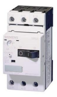
CIRCUIT-BREAKER, SIZE S00, FOR MOTOR PROTECTION, CLASS 10, A REL.0.45...0.63A, N REL.8.2A SCREW CONNECTION, STANDARD BREAKING CAPACITY, W. TRANSV. AUX. SWITCH 1NO/1NC
