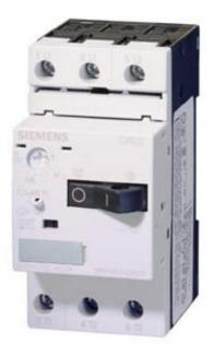
CIRCUIT-BREAKER, SIZE S00, FOR MOTOR PROTECTION, CLASS 10, A REL.0.35...0.50A, N REL.6,5A, SCREW CONNECTION, STANDARD BREAKING CAPACITY W. TRANSV. AUX. SWITCH 1NO/1NC
