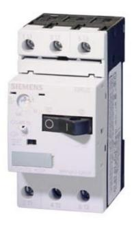
CIRCUIT-BREAKER, SIZE S00 FOR MOTOR PROTECTION, CLASS 10, A REL.0.14...0.2A, N REL.2.6A, SCREW CONNECTION, STANDARD BREAKING CAPACITY W. TRANSV. AUX. SWITCH 1NO/1NC
