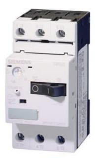
CIRCUIT-BREAKER, SIZE S00, FOR MOTOR PROTECTION, CLASS 10, A REL.0.55...0.8A, N REL. 10A, SCREW CONNECTION, STANDARD BREAKING CAPACITY W. TRANSV. AUX. SWITCH 1NO/1NC
