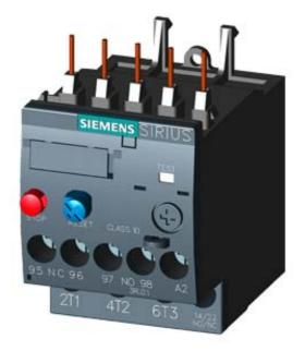
OVERLOAD RELAY 9.0...12.5 A FOR MOTOR PROTECTION BGR S00, CLASS 10 FOR MOUNTING ONTO CONTACTORS MAIN CIRCUIT: SCREW TERMINAL AUXILARY CIRCUIT:SCREW TERMINAL MANUAL-AUTOMATIC-RESET
