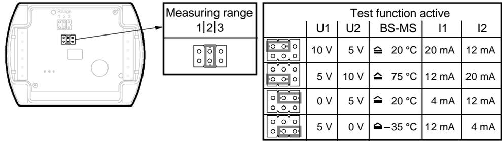
The setting element is located inside the cover. It comprises 6 pins and a jumper. It is used to select the required measuring range and to activate the test function.
