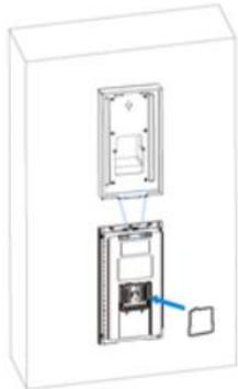
For convenient wiring, hang R27X on the wall-mounting box/flush-mounting bracket with rope. Then insert the silicon rubber sealing ring into the groove.
