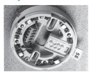
The EBI-11 isolating base senses and isolates short circuit faults on FX Fire Detection Panel loops and is intended for use with Intellia detectors.
