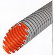
A flexible, halogen-free electrical installation conduit made of a special light grey (RAL 7035) plastic material, with an orange inner gliding layer.
