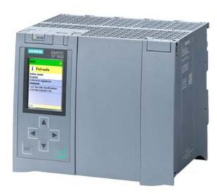
SIMATIC S7-1500F, CPU 1517F-3 PN/DP, CENTRAL PROCESSING UNIT WITH WORKING MEMORY 3 MB FOR PROGRAM AND 8 MB FOR DATA, 1. INTERFACE, PROFINET IRT WITH 2 PORT SWITCH, 2. INTERFACE, ETHERNET, 3. INTERFACE, PROFIBUS, 2 NS BIT-PERFORMANCE, SIMATIC MEMORY CARD NECESSARY
