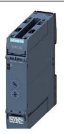
TIMING RELAY, ELECTRONIC, OFF-DELAY, WITHOUT CONTROL SIGNAL OR NON-VOLATILE RELAY DEFINITE PASSING MAKE CONT., 24 V AC/DC, 1 CO CONTACT 7 TIME SET. RANG. 0.05S...600S, WITH LED, SCREW TERMINAL
