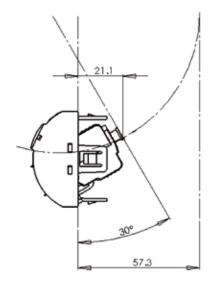
Minimum Depth using Brand-Rex UM-10 Cable. (Minimum Cable Radius = 8 x Cable Dia)
