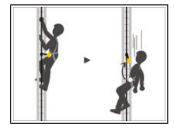
For vertical progression with a rail or cable-based fall protection system, the LADDER CLIMB attachment point allows for ventral attachment of the trolley, which distributes the load on the waistbelt and thus ensures optimal comfort. In case of a fall, this attachment point automatically moves upward to a sternal position to ensure a vertical post-fall body position.
