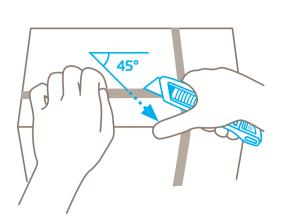
Use the slider to **engage the blade** for cutting.
