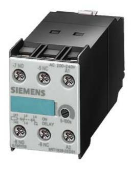
SOLID-STATE, TIME-DELAYED AUXILIARY SWITCH BLOCK SETTING RANGE 5 S...100 S, AC 100...127 V, 1NO + 1NC, ON-DELAY, FOR MOUNTING ONTO CONTACTORS SIZE S0...S12
