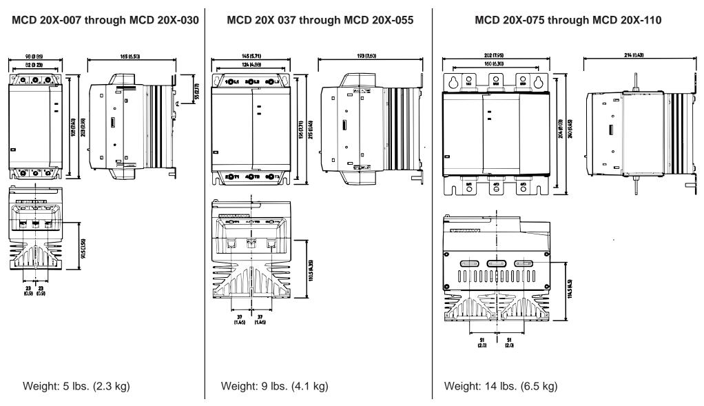
All units suitable for operation on input voltages from 200 through 480 volts
