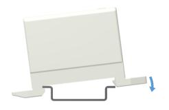
**DIN-rail mounting**Set the connector to DIN-rail.
