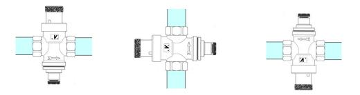
The pressure reducers MINIBRASS don't get the effects, in their functioning, of gravity force; therefore they can be installed in the plant in any position:
