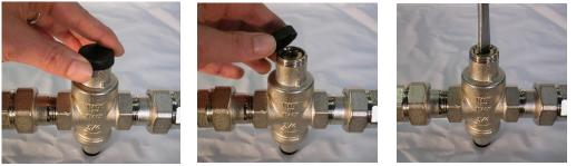
All Malgorani pressure reducers are tested before being packaged; during the test they are set at the outlet pressure of 3 bars; outlet pressure can be easily adjusted once the pressure reducing valve in installed on site.
