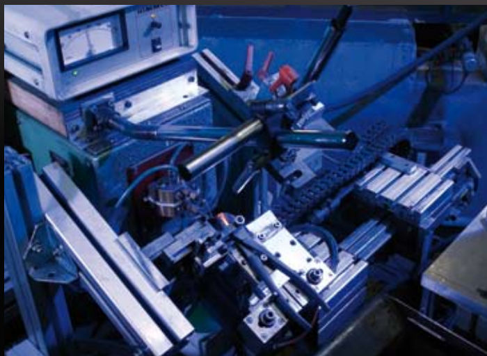
Optimum bonding between the coating and the pliers blank is ensured through the use of special assembly fixtures combined with dispensing units for adhesives.
